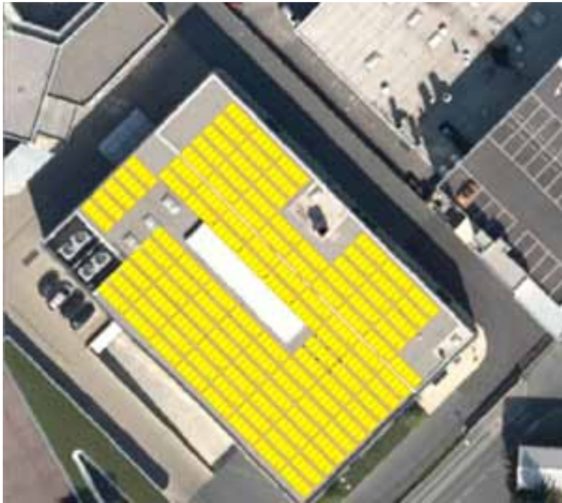
Figure 66 - Second roof with directly on roof mounted collectors
